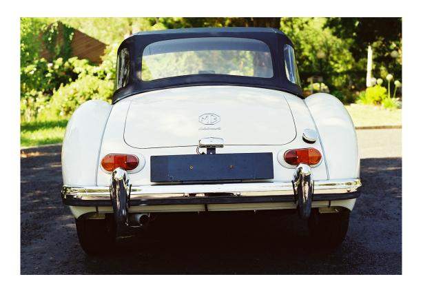
(As incidentally can be seen in the above illustration, all of the Australian assembled MGA cars took the wiring for the number plate light around the rear valence panel, rather than (more neatly) through it as in their UK counterparts.)
